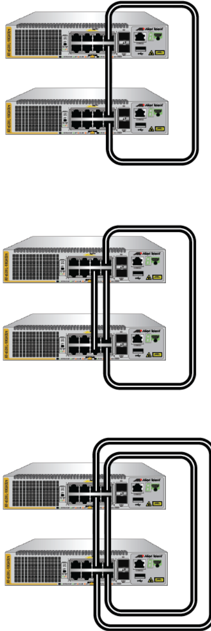
Figure 28. Trunks of 5Gbps Ports for Stacks of Two x530L-10GHXm Switches
