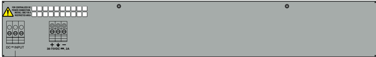
Figure 2: DC Power inlet terminals on an AT-8724XL.
